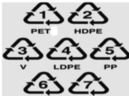
Figure - 7 PET-Polyethylene terephthalate, HDPE-Highdensity polyethylene, V-Vinyl (PVC), LDPE-Low density polyethylene, PP-Polypropylene, PS-Polystyrene and Other means all other resins and multi-materials like ABS, PPO, PC, PBT. Source – Plastic Waste (Management and Handling) Rules, 2011.
